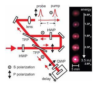
FIG. 2. (Color online) Setup showing the DPI. QWP=quarter-wave-plate; HWP=half-wave-plate; TFP=thin film polarizer. The right panel shows beam images of filamentation and white light generation for increasing pulse power up to  $\sim 2.8 P_{\rm cr}$ .
