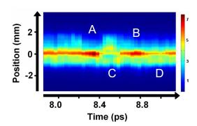
FIG. 5. (Color online) As in Fig. 4(a), 1D integrated images of the probe filament as a function of delay near t=8 ps but with no pump/probe misalignment. Pump/probe energies are 3.6 mJ/4.6 mJ ( $2.8P_{cr}/3.6P_{cr}$ ). Note the funneling of laser energy from the reservoir into the filament at location A and the expulsion of filament light at location B.
