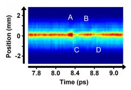
FIG. 6. (Color online) 1D integrated images of the probe filament aligned with a parallel polarized pump filament as a function of delay near t = 8 ps. The pump and probe are perfectly collinear and each have energy of 3.3 mJ (2.6 $P_{ct}$ ).
