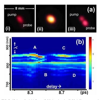
FIG. 7. (Color online) (a) Pump  $(2.3P_{cr})$  and probe  $(2.5P_{cr})$  filament central spots in far field with initial ~0.1 mrad misalignment, where (i) probe delay is detuned from revivals, (ii) probe is delayed to location A in Fig. 4(a), and (iii) probe is delayed to location C in Fig. 4(a). (b) Probe filament spectrum as a function of delay (33 fs steps) through the air alignment revival near t=8 ps.
