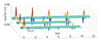
FIG. 1. (Color online) Measured alignment of 1 atm of N<sub>2</sub> and O<sub>2</sub> at room temperature (295 K) by a 110 fs, 800 nm,  $4.1 \times 10^{13}$  W/cm<sup>2</sup> laser pulse. The effective alignment of air is synthesized from the N<sub>2</sub> and O<sub>2</sub> plots.
