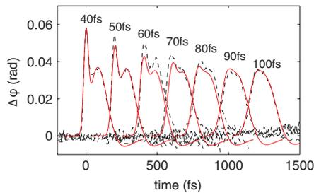
FIG. 3. (Color online) Pulse-width dependence of the nonlinear response in  $N_2$ . Measured phase shift extracted using SSSI (black dashed line), with the pulse width varied between 40 and 100 fs by adjusting the compressor. The pulse energy is kept constant. Also shown is the phase shift calculated (red solid line) using Eq. (1) and the parameters ( $n_2$ ,  $\Delta\alpha$ ) measured with a 40-fs pulse.
