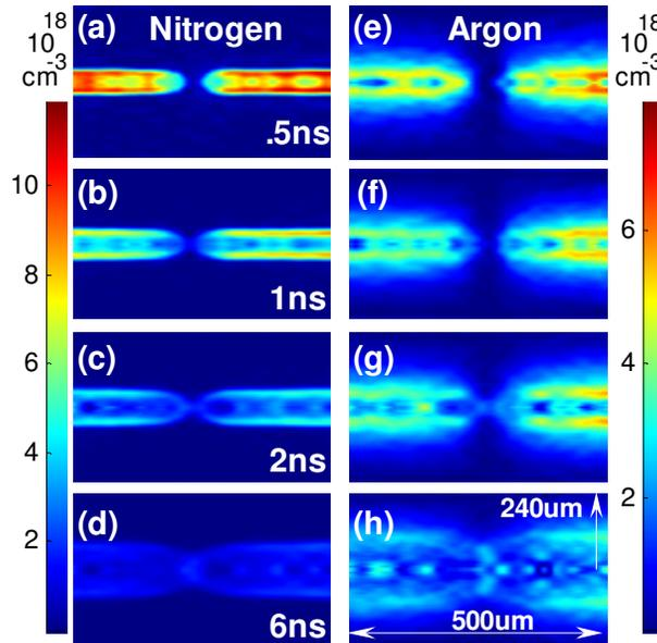
Fig. 2. Waveguide electron density profiles at indicated delays vs. radius and axial position produced in nitrogen (a-d) and argon (e-h) cluster jets at 800 psi backing pressure and  $-145^\circ\text{C}$  ( $22^\circ\text{C}$ ), with single 25  $\mu\text{m}$  diameter wire across the exit of the elongated nozzle and in contact with it. Channels were formed using a Nd:YAG pump (1064 nm, 500 mJ, 100 ps).
